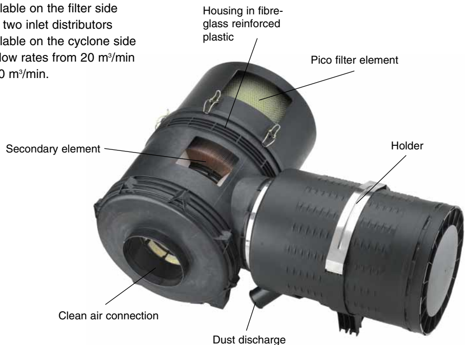
NLG Pico version with DualSpin® pre-separator
