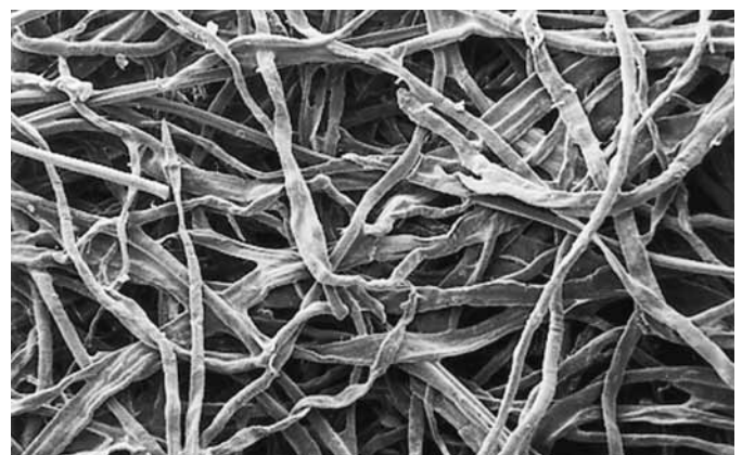
A microscope scan of the CompacPlus® filter medium
