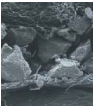
Microscopic view: Activated charcoal embedded in nonwoven
